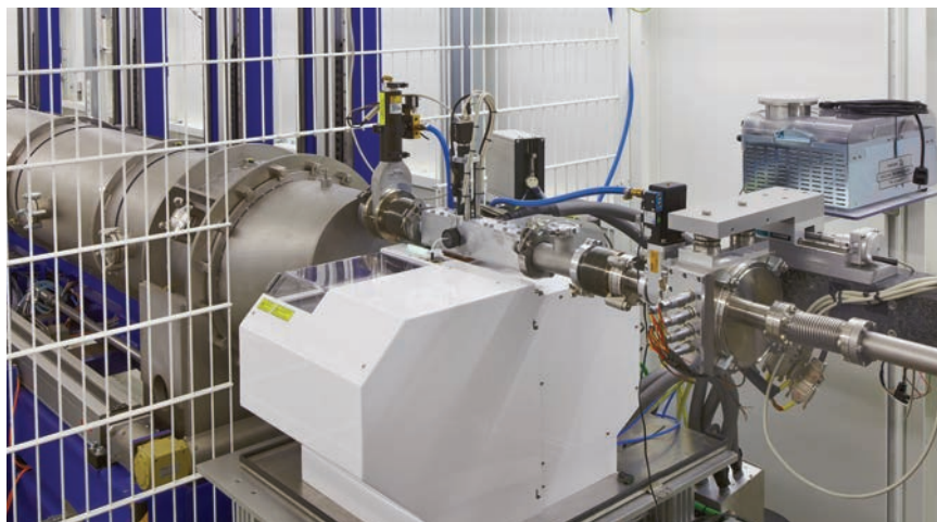
The new sample changer on the Bio-SAXS beamline at EMBL Hamburg
