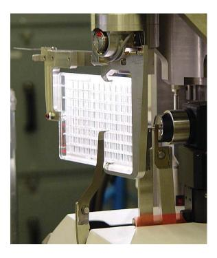
Micro-crystals in situ data collection – CD plate mounted on a MD3 diffractometer, at the EMBL@PETRA3 P14 beamline.
