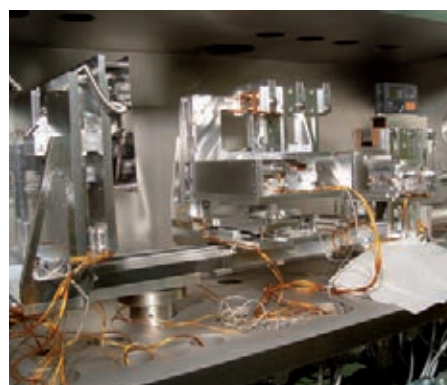
The multilayer monochromator in its vacuum vessel during installation at beamline BW7A. From right to left (beam direction), first and second multilayer located on their respective positioning devices and the slit system with integrated intensity monitor are shown
