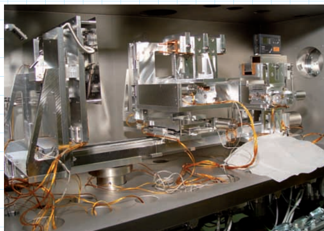
The multilayer monochromator in its vacuum vessel during installation at beamline BW7A. From right to left (beam direction), first and second multilayer located on their respective positioning devices and the slit system with integrated intensity monitor are shown.
