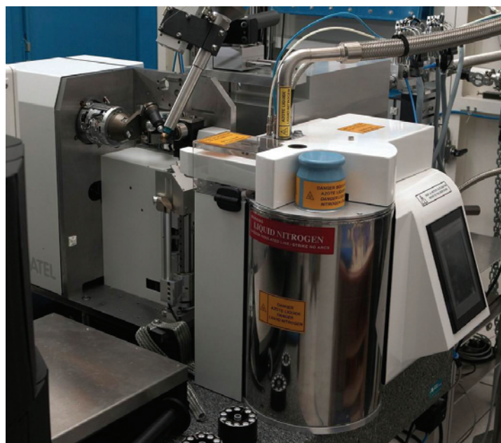
MD2M diffractometer and SC3 sample changer.
