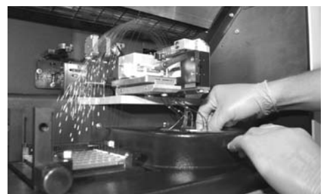
A bundle of capillaries used to analyse most sequenced samples at GeneCore.
