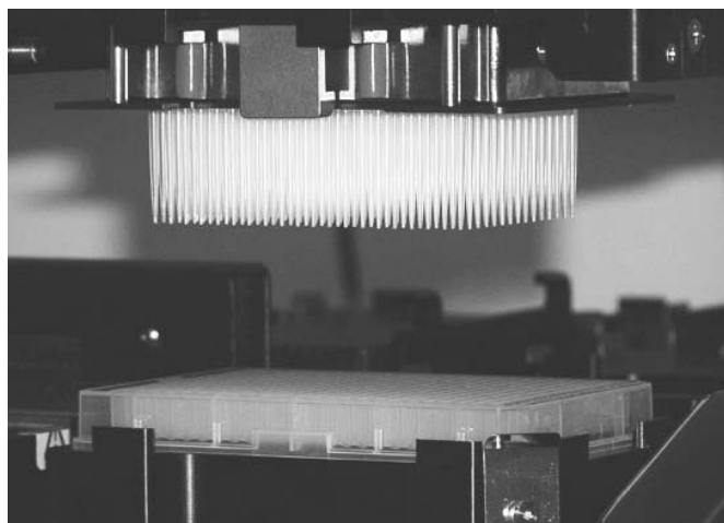
Parallel pipetting of samples in 384-well format.
