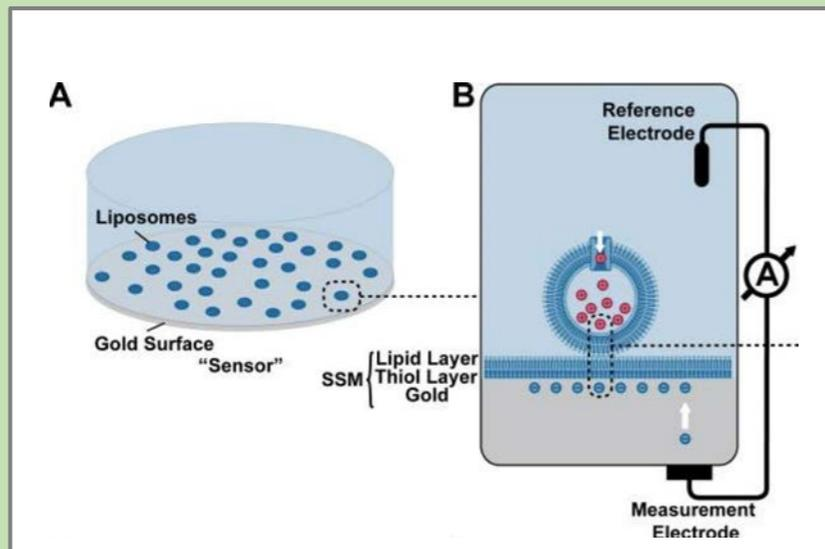
**Figure 5. SSM electrophysiology setup.** A. Liposomes with reconstituted protein are adsorbed on the thiolized gold sensor. B. Changes in electrical potential are detected that are generated by electrogenic transport. Figure adapted from Barthmes et al., 2016<sup>5</sup>
