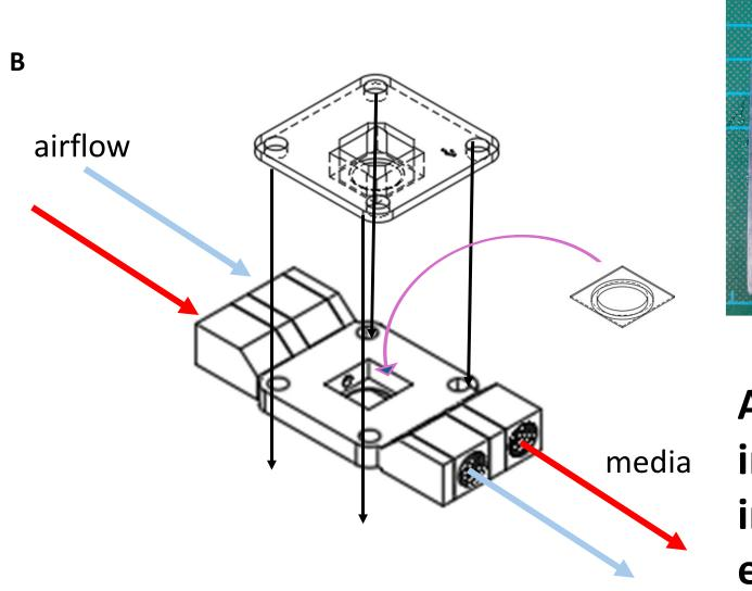
A) The nasal OoC device parts, constructed device, and three possible lids to create different airflows onchip, B) the mode of construction of the nasal device, C) resin printed device for higher throughput of perfusable inserts, using interference fit with soft printed insert holder.
